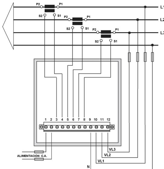
Three-phase networks - 4 wires (low voltage)
