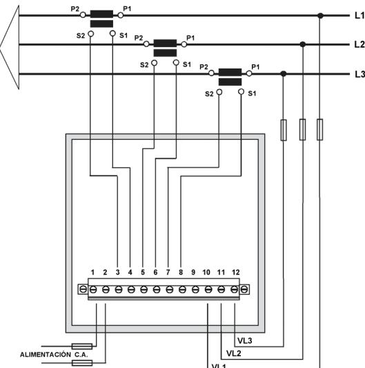
Three-phase networks - 3 wires (low voltage)
