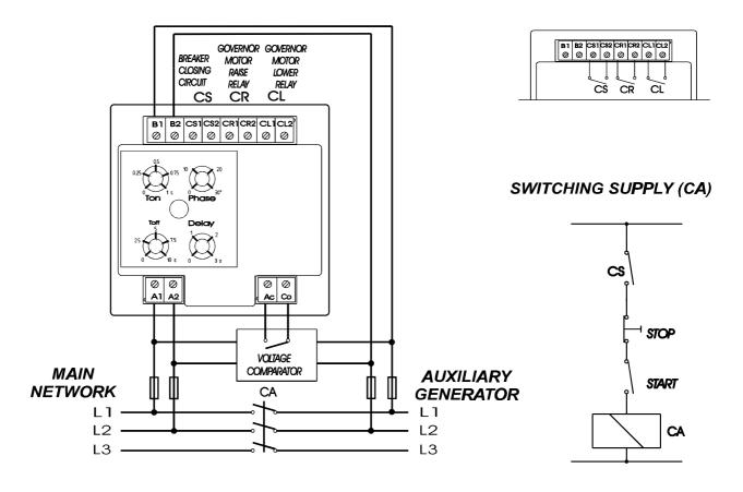
\* LINK AC AND CO TERMINALS IF VOLTAGE COMPARATOR IS NOT REQUIRED
