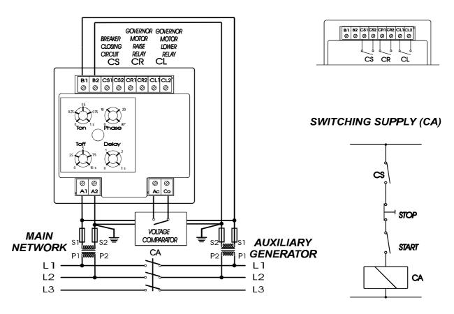
\* LINK AC AND CO TERMINALS IF VOLTAGE COMPARATOR IS NOT REQUIRED
