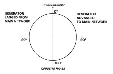
Actually, when the phase shift between generator voltage and mains voltage is close to 0, the zone (3) is lit on.
