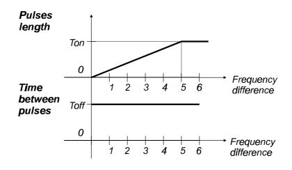
Examples: Adjusted times:  $T_{off}$ = 4 s and  $T_{on}$ = 1 s
