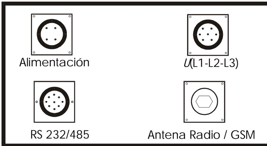
The **QNA-303** analyzer is equipped with a RS communication port to set the communication to the PC. The connection arrangement will depend on the communication mode to be used.
