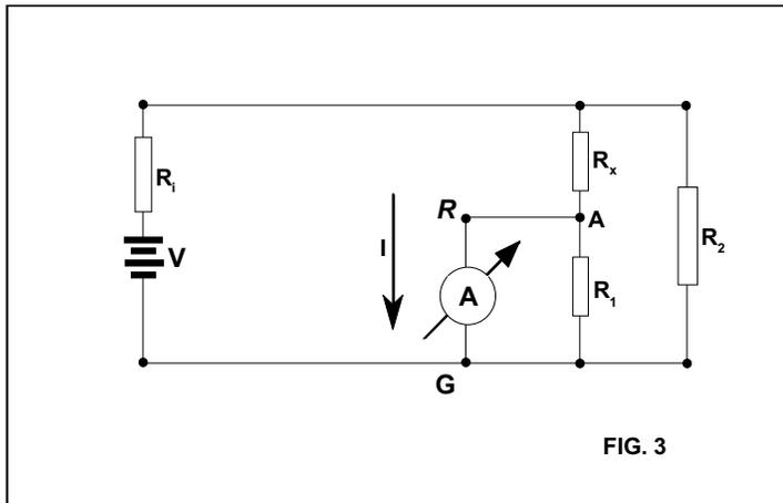
In the circuit of Fig. 3 it may be noted that R1 is in parallel with a low-value resistance (the one of the microammeter) therefore its influence is minimized during reading.
