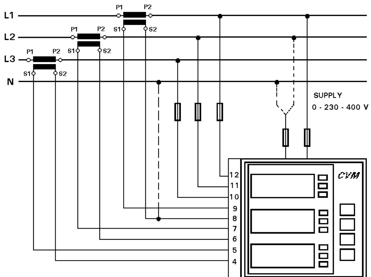
**NOTE :** FOR A HIGH VOLTAGE NETWORK IS ALWAYS ADVISABLE TO INSTALL THE CVMk - ITF... (isolated current inputs).
