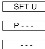
Last digit of the first display indicates "U" (Voltage) and first digit of the second display indicates "P" (Primary). It means that we can set the primary of the voltage transformer. To avoid mistakes the Voltage red LEDs remain lit on.
