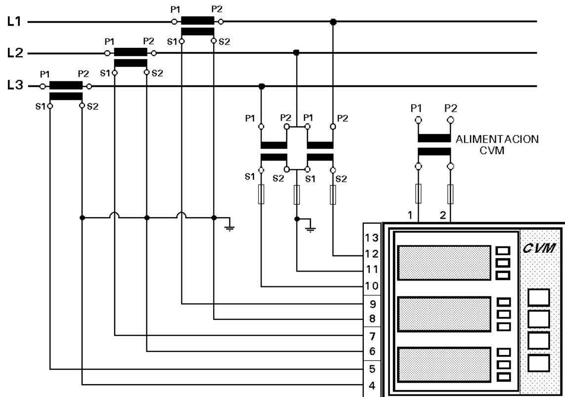
C.- **CVMk-ITF** : Two current transformers + 2 voltage transformers.
