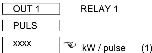
(1) Value of energy in kW : four digits with floating decimal point
