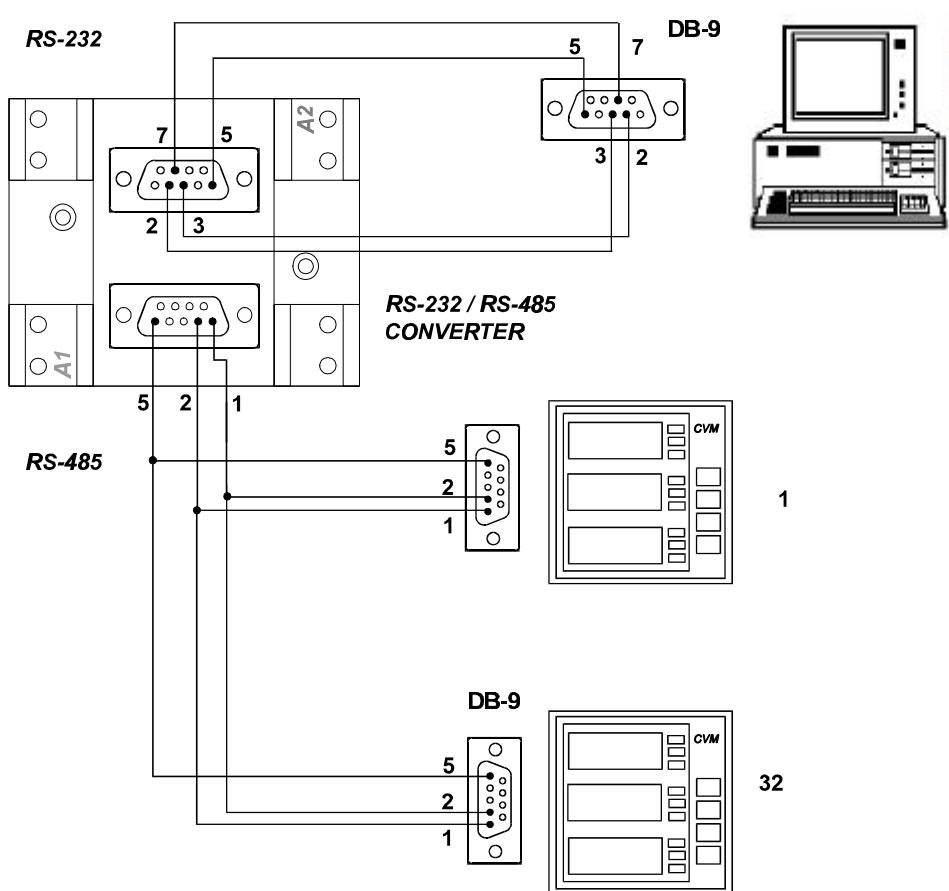
RS-485 connection will be carried out by means of a **twisted and screened cable**, with a minimum of 3 wires, with a maximum distance between the CVMk and the last peripheral of 1.200 m. The CVMk with the CVM/xxx485 module uses a RS-485 communication bus allowing up to **a maximum of 32 devices in parallel (Multidot bus) per used port of the PC**.
