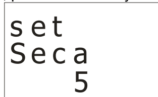
Figure 33. Current secondary value I_N/5A
