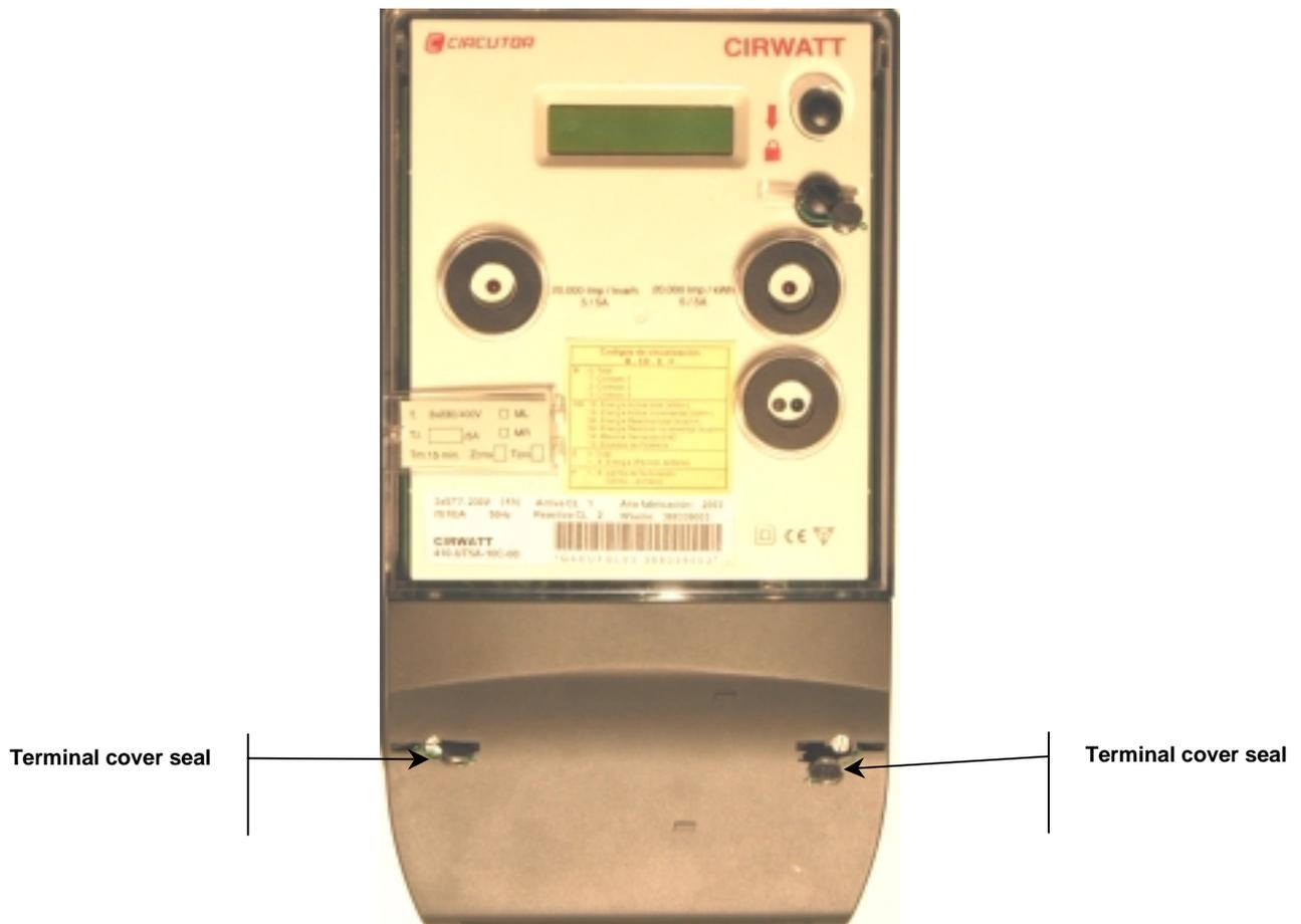
Changing the clock battery is protected by this seal.
