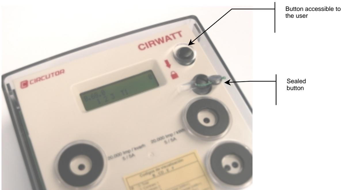
They operate by using the short press-long press system. A short press is one that lasts for less than 2 seconds. While a long press lasts more than 2 seconds
