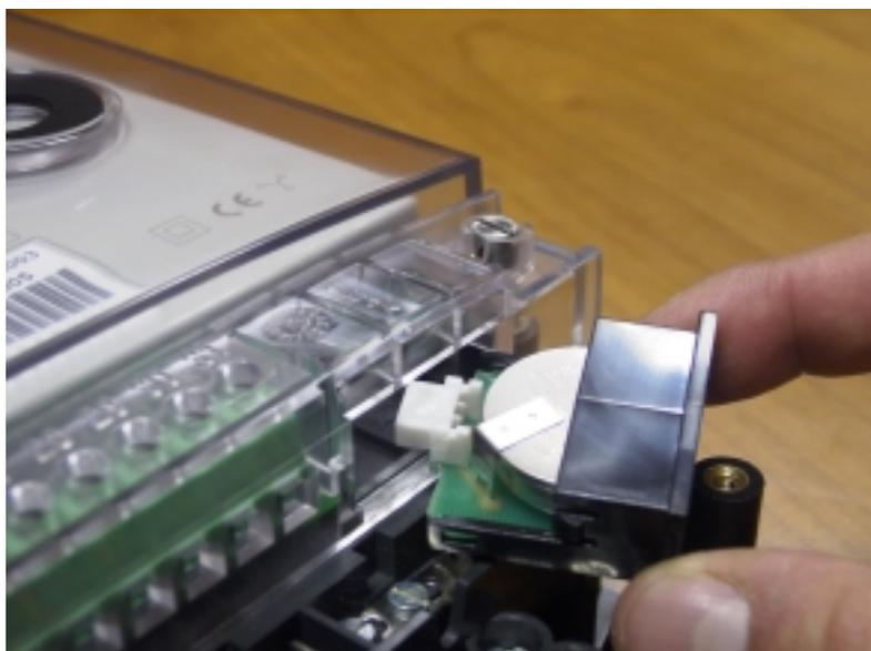
It is noted that the battery can be replaced with the meter receiving voltage, because there is no contact at any time with dangerous voltages.
